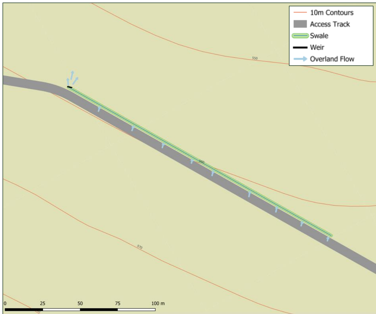
Plate 1: Concept Swale Design for Access Track Sections <1V:3H
